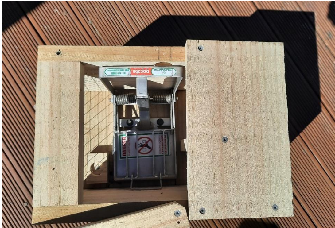
Figure 16 DOC200 trap box fixed partial lid design.
